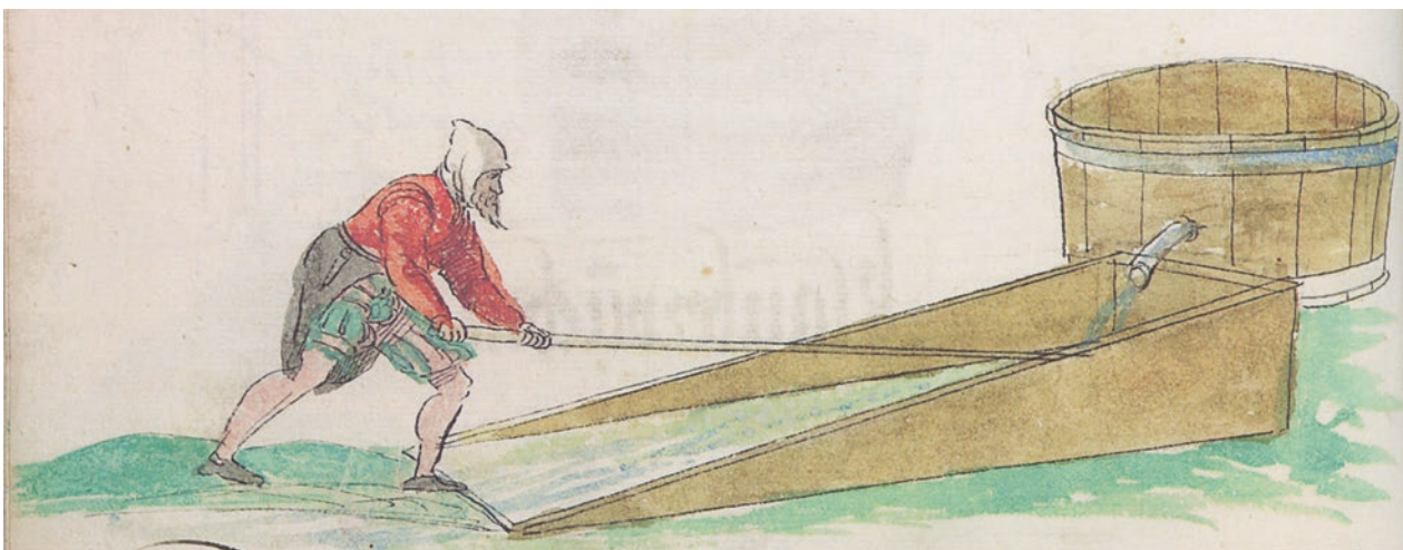
Fig. 4.0-32: Schwazer Bergbuch : Installation for ore washing (after Bartels et al. 2006, 150).
