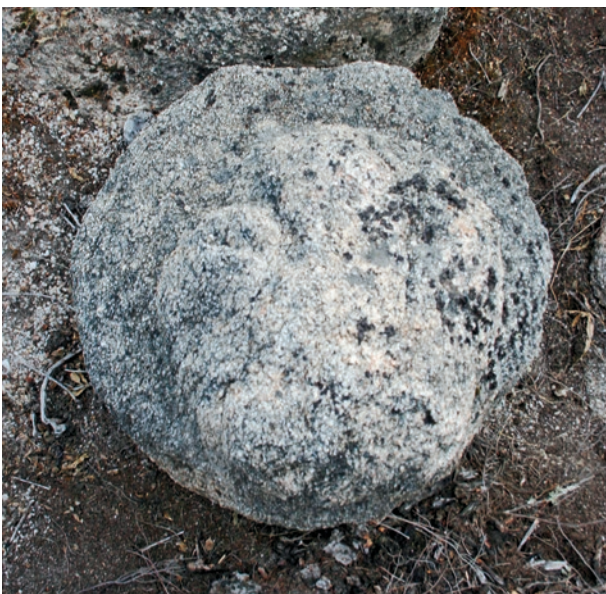
Fig. 6.0-19a/b: Territorium metallorum Tresminas / Jales, Fonte da Ribeira quarry: the stone had to be discarded during straightening of the opposite side due to the fissures. Diameter 42 cm, H max. 38 cm, projected height at the end 19 cm (photo a: R. Wahl-Clerici, photo b: T. Schierl).
