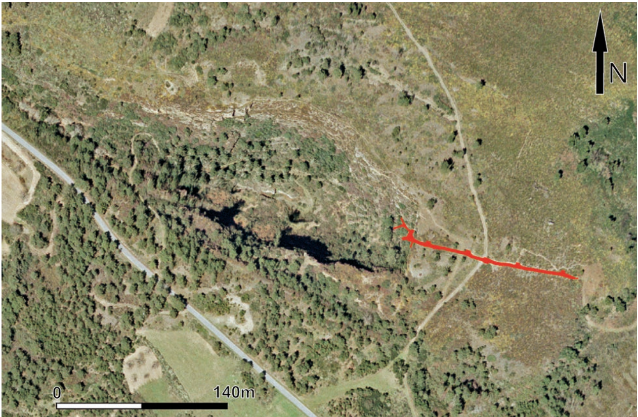
Fig. 3.3-26: Territorium metallorum Tresminas / Jales, Tresminas, Galeria dos Alargamentos: at the point where the two tunnels meet, an unintentional extension is visible, demonstrating that the two tunnels did not meet exactly head on (Ortofotomapa 1:5000 Câmara Municipal de Vila Pouca de Aguiar; measurement, processing and presentation M. Helfert).
