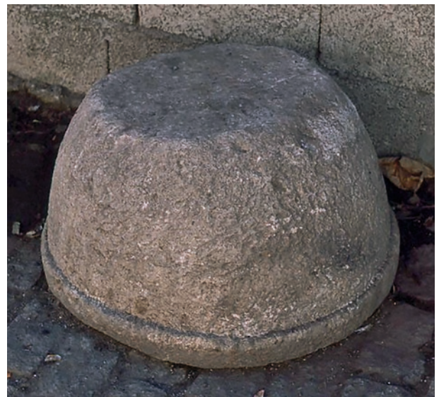
Fig. 4.0-26: Territorium metallorum Tresminas / Jales, Tresminas: surface find of a sleeper from a different mill-type for further milling the stamped ore (photo: R. Wahl-Clerici).
