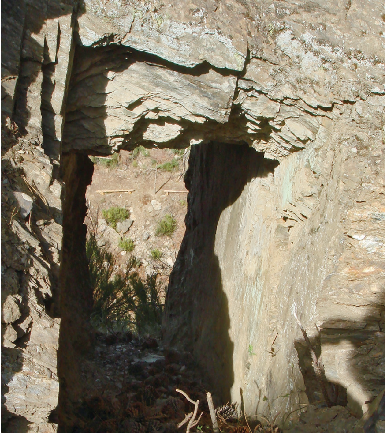
Fig. 3.1-6: Territorium metallorum Tresminas / Jales, Tresminas, Corta de Covas: stairwell for prospection. For the eastern wall, a natural fissure was used (photo: R. Wahl-Clerici).
