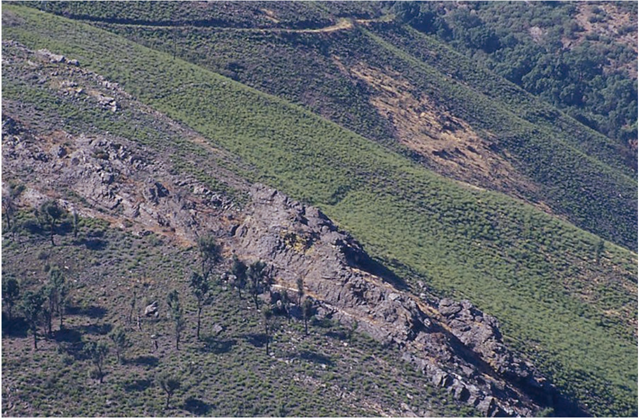
Fig. 5.0-26: Territorium metallorum Tresminas / Jales: the marked ridge in the slope shows the course of the aqueduct C4, which continues in the rock cut in figs. 5.0-27a/b/c, 5.0-28 (photo: J. Wahl).
