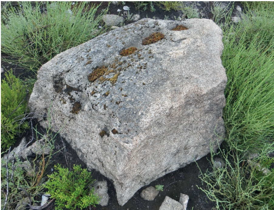
Fig. 6.0-7: Territorium metallorum Tresminas / Jales, Fonte da Ribeira quarry: block prepared for splitting, from which parts have already been split off at the front and side (photo: R. Wahl-Clerici).
