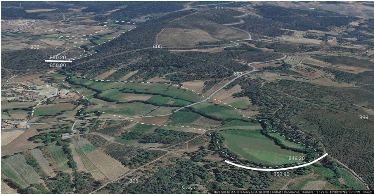
Fig. 5.0-6: Territorium metallorum Tresminas / Jales: schematic overview of the Outeiro and Sainça dams and their highest possible water level (template Google Earth, 14.12.2015, inclination with viewing height of 1.19 km, design: R. Wahl-Clerici).
