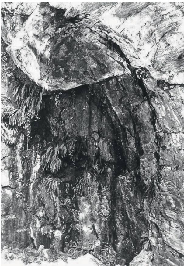
Fig. 3.1-11: Territorium metallorum Tresminas / Jales. Tresminas, Corta de Covas: remains of fire-setting with the typical dome shaped traces in the rock (photo: J. Wahl).
