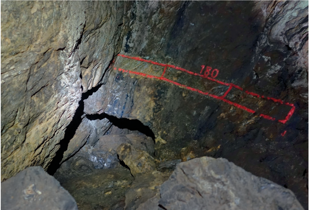
Fig. 3.0.1-11: Territorium metallorum Tresminas/Jales, Lagoinhos: the sample in nr. 180 is sterile, below are the prospections PR-2 and PR-4. View towards the east-end of the mining area. (R. Wahl-Clerici).
