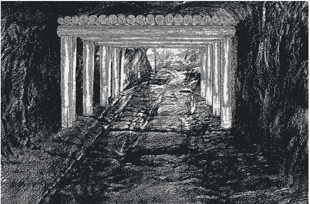
Fig. 3.3-31: Territorium metallorum Tresminas / Jales, Tresminas, Corta da Ribeirinha, Galeria dos Morcegos: the reconstruction of the timber posts is based on the cuts in the rock of the floor (drawing: P. Moser).
