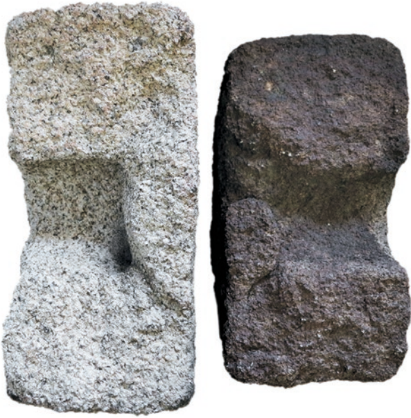
Fig. 6.0-21: Territorium metallorum Tresminas / Jales, Fonte da Ribeira quarry: runner with incorrectly positioned central hole, broken in two halves. Diameter max. 42,5 cm, diameter central hole min. 7,5 cm, max. 10,5 cm, H max. 19 cm (photo: R. Wahl-Clerici).
