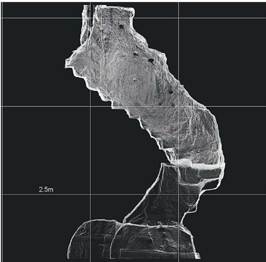
Fig. 2.2-7: Territorium metallorum Tresminas / Jales. Tresminas, Corta da Ribeirinha: section through the point cloud of the stairwell of the U-shaped staircase; view from east. The steps are clearly visible as are the steps in the ceiling and the connecting shaft to the Galeria do Pastor (recording and imaging: K. Mechelke, M. Lindstaedt).
