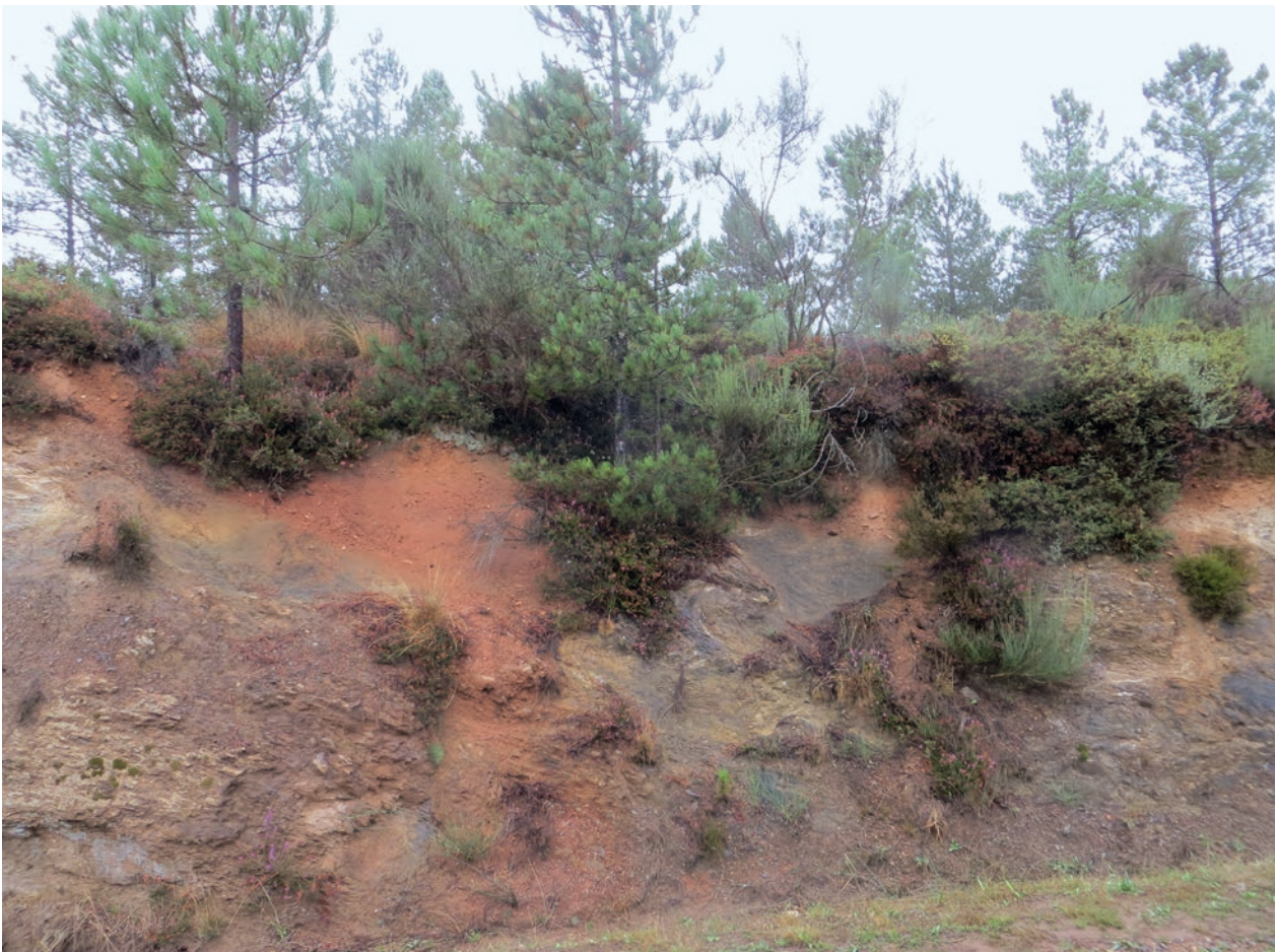
Fig. 5.0-14: Territorium metallorum Tresminas / Jales: pit on the road from Tinhela de Baixo to Tresminas, where the typical reddish, loamy material that was used to build the earth fill dams, is visible (photo: R. Wahl-Clerici).
