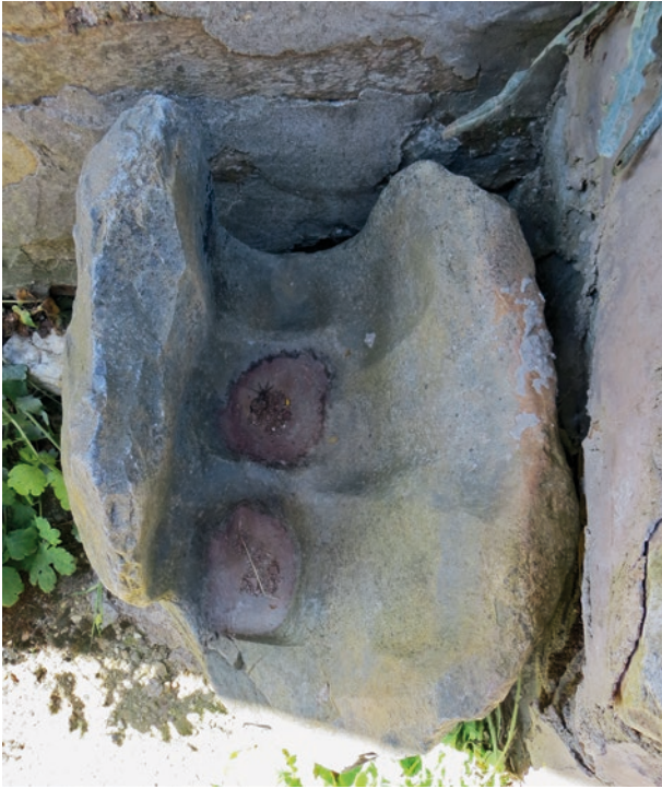
Fig. 4.0-20: Pozos (Prov. León / E): heavily used stamp mill base for at least three stamps (photo: R. Wahl-Clerici).
