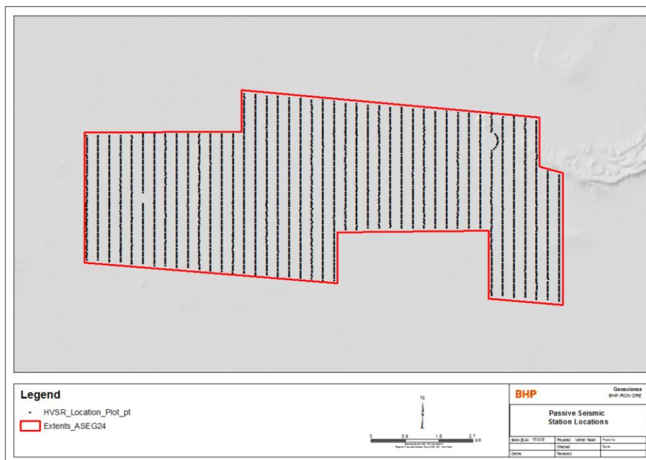
Figure 3. Plot of actual passive seismic geophone locations/ stations (black). Survey extents shown in red. Note that coordinates have been deliberately omitted.
