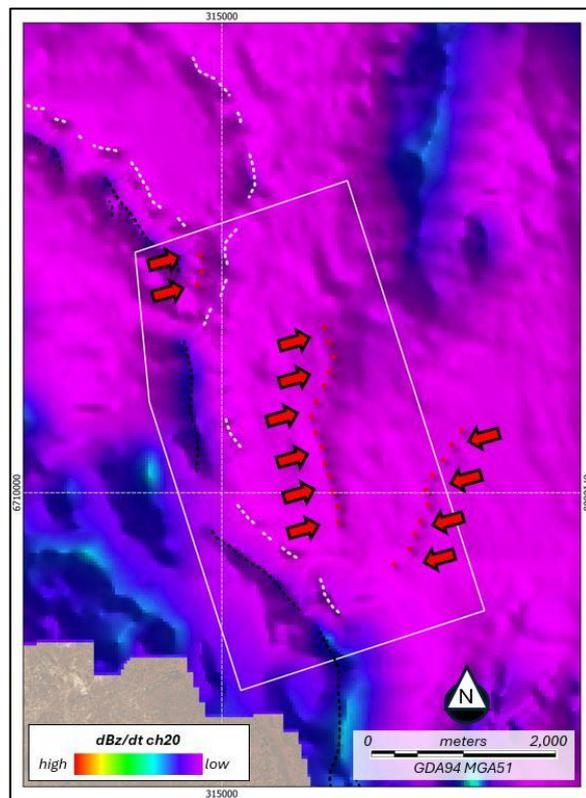
Figure 2. Mid-time AEM data (dBz/dt ch20 – 2.12ms) over the Springfield prospect (white rectangle). Interpreted stratigraphic conductors are depicted with black and white dashed polylines. The red arrows point to semi-linear areas of suspected IP effect expressed as a trough in the mid-time channel AEM data.
