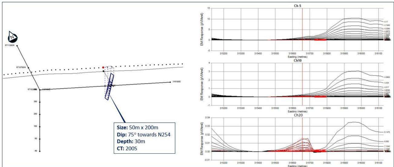
**Figure 4. Left: Thin EM plate modelled from IP-corrected AEM dBz/dt data tested by drillhole SFRC16. Right: IP-corrected AEM dBz/dt data profile in black and plate model response in red along line 10470.**
