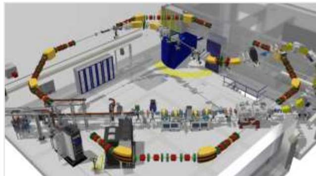
Figure 52: cSTART, with 14 m diameter, producing ultrashort X-rays [from the talk of M. Fuchs].
