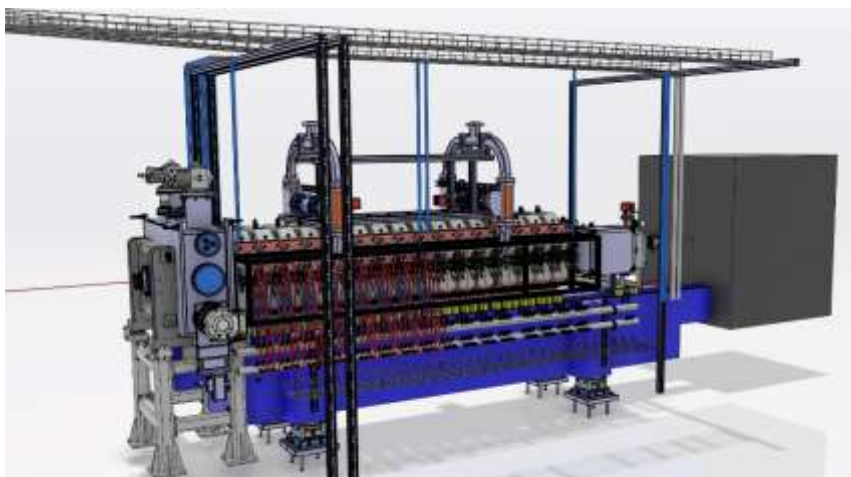
Figure 24: The FCC-ee PoP e+ source at PSI (P3) with HTS solenoid as adiabatic capture device [from the presentation of I. Chaikovska].
