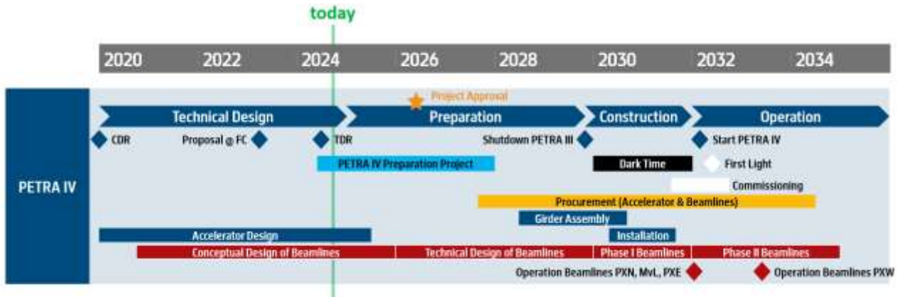
Figure 31: Time line of PETRA IV [from the presentation of I. Agapov and R. Bartolini].
