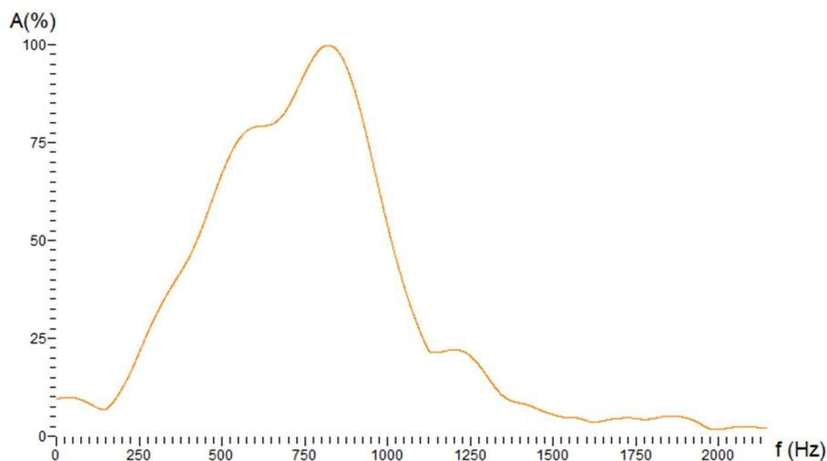
**Figure 3. Signal spectrum of the sparker source on the source depth (100 m) in the injection well (Brumbys-1) from the last monitor (post-injection) data**
