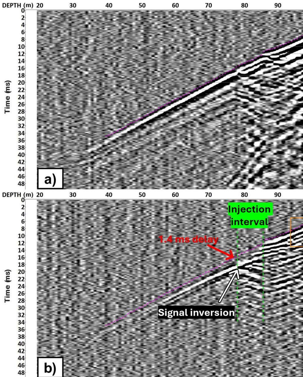
Figure 2. Brumbys-3 (injection well) data: baseline acquired a day before injection (a) and last monitor acquired two days after injection (b) for 100 m depth source position. The purple line shows direct wave travel time for baseline data. The red arrow points first breaks delay after the end of the injection. The orange rectangle shows the signal spectrum estimation area for Figure 3.
