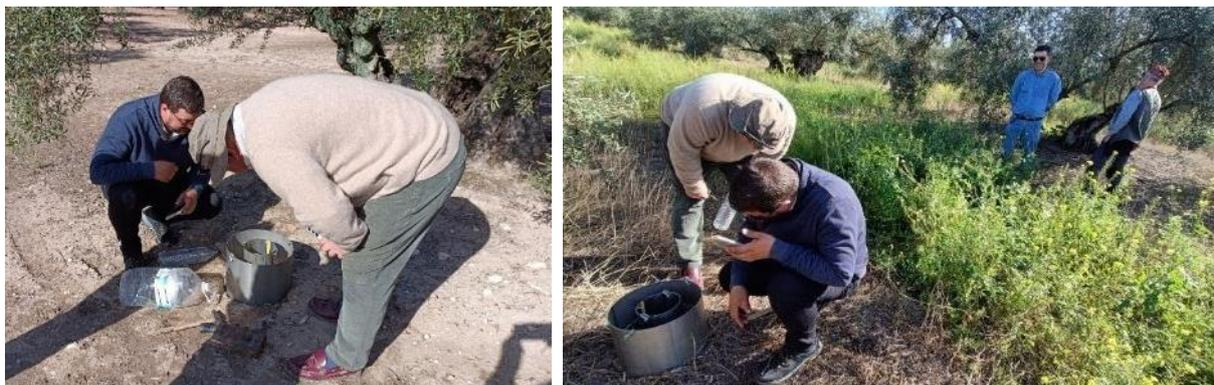
**Figure 15.** Demo of water infiltration test in the field.
