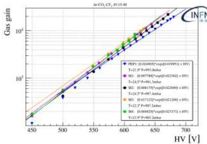
**Fig.4.3** Gas gain calibration for different  $\mu$ -RWELL prototypes: (blue) 10x10 cm<sup>2</sup> from D7.3 report (black) 30x25cm<sup>2</sup> from this report.
