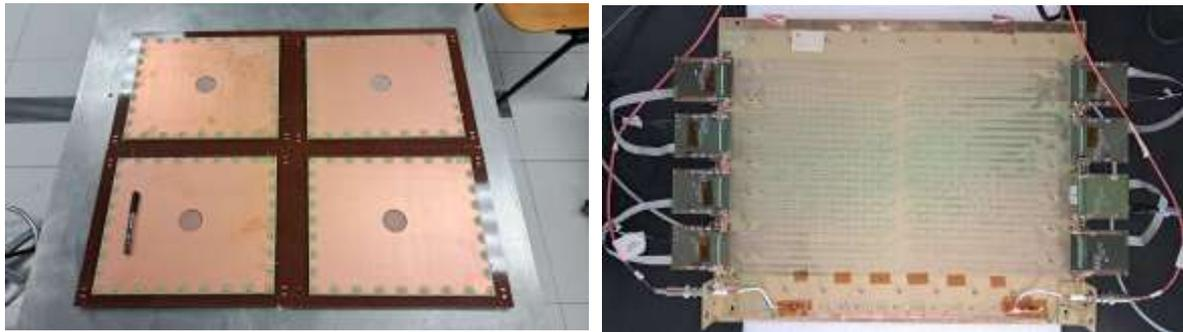
**Fig.3.2** (left) the four 30x25 cm<sup>2</sup> detector produced, picture from the cathode view (right) picture of a single detector from the backplane view: the R/O routing and the FEE instrumentation are visible.
