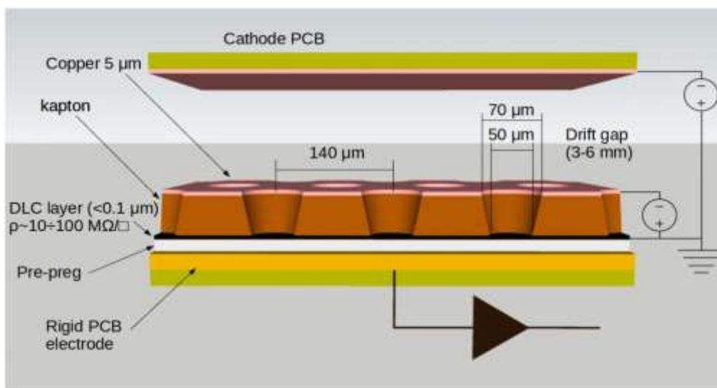
**Fig.2.1** Basic layout of a  $\mu$ -RWELL
