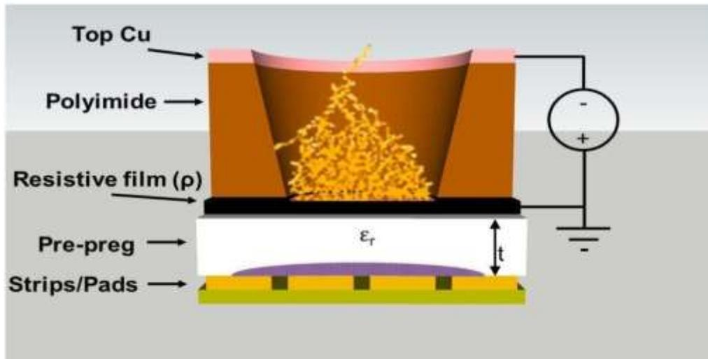
**Fig.2.1** Principle of operation of a  $\mu$ -RWELL
