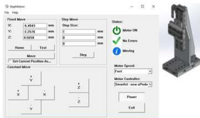
Figure 5: The two piezo-stages at the DuMi end-station are controlled with the developed StepMotion software incorporated in SPECTOR.
