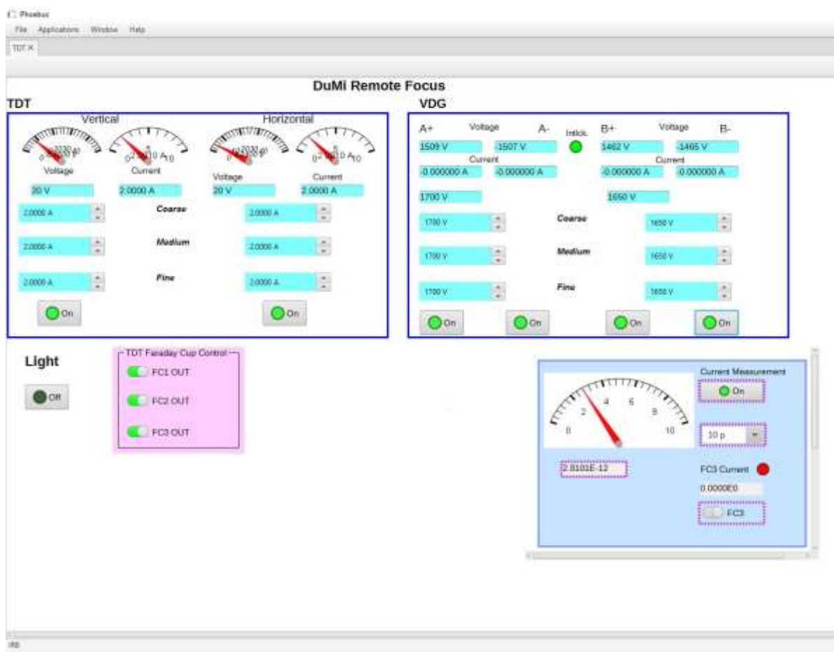
Figure 9: The ion beam focusing in the DuMi setup is remotely controlled through EPICS. Faraday cups as well as ion beam current reading is also obtained in the same way.
