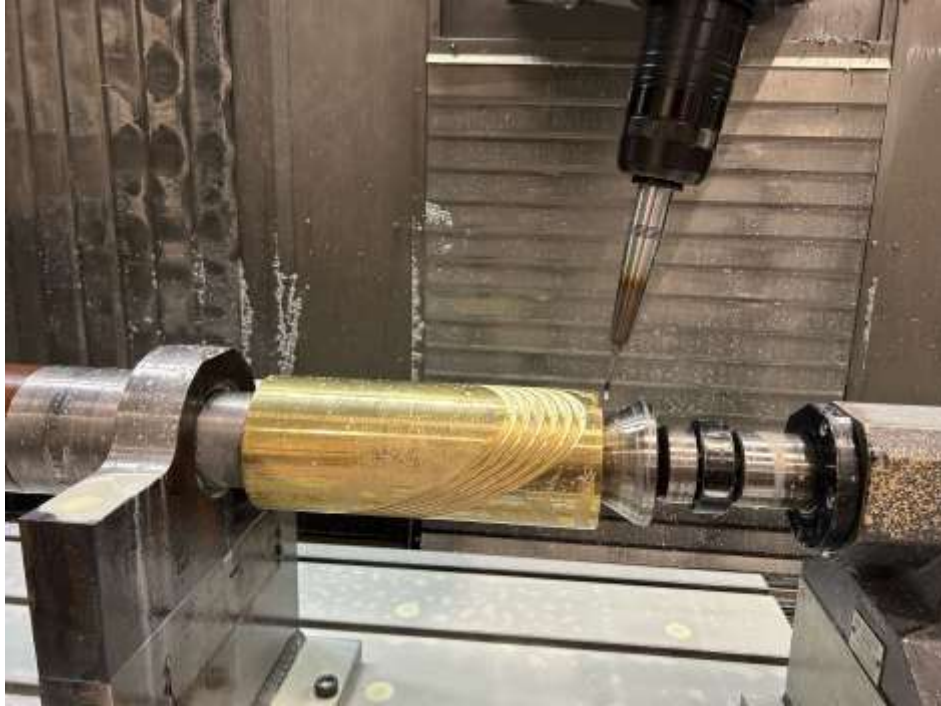
Figure 5: Manufacturing of the test former at https://hsm.as
