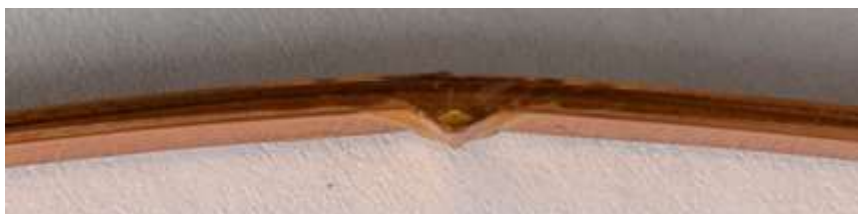
Figure 2: Behaviour of a Cu tape stack insulated by a commercial self-adhesive kapton tape
