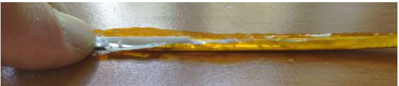
Figure 10: Wax observed inside the kapton insulation after opening it up
