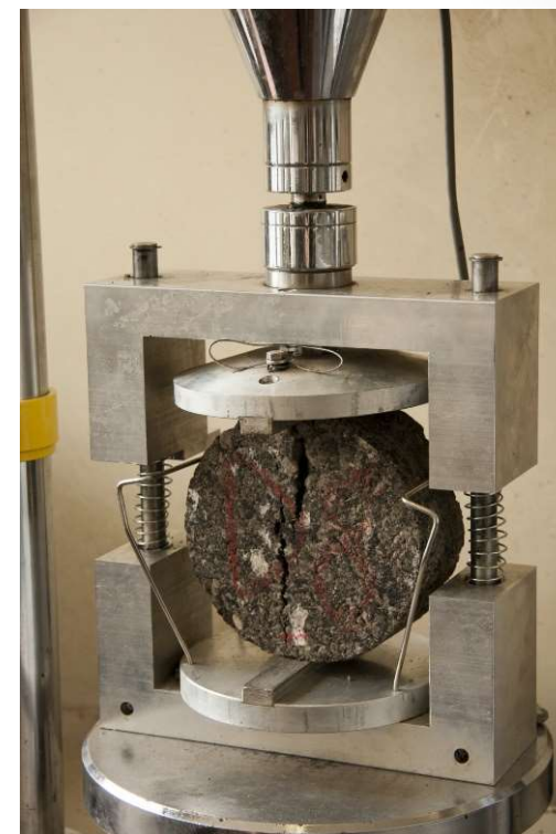
Indirect tensile strength test (destructive) @15°C
