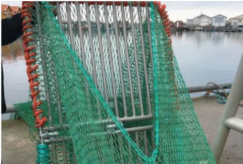
Figure 9 Fishing gear for Nephrops with grid and opening for bycatch.
