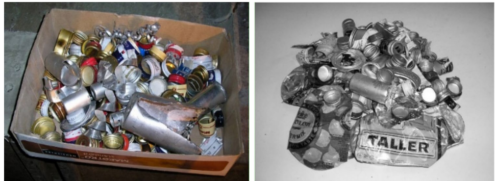
Figure 1 Remelted waste of thin-walled aluminium charge with a developed surface (for example, cans for various drinks).
