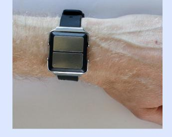
PulseOn Arrhythmia Monitor Continuous PPG. Vibrated 4 times per day and upon irregular pulse to prompt ECG recording.
