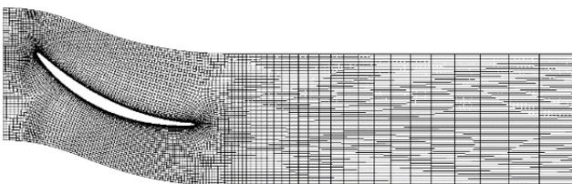
**Figure 4 : A sample of S2 mesh treatment used to reduce the wave reflection.**
