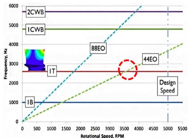
Figure 1 : Campbell Diagram of Purdue configurations. The 1<sup>st</sup> torsion mode shape of R2 blade is plotted.
