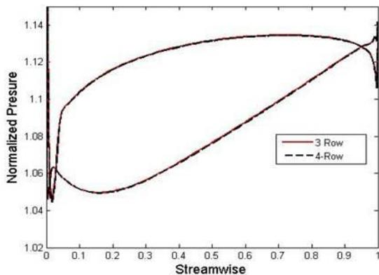
Figure 8 : R2 time-averaged blade loading comparison across different extended domain cases.
