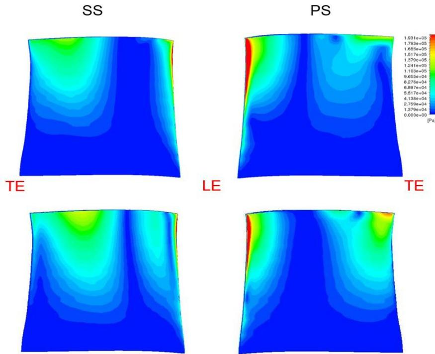
Figure 7 : Modal force distribution on R2 blades. Three-row simulation is on the top and the 4-row case on the bottom.
