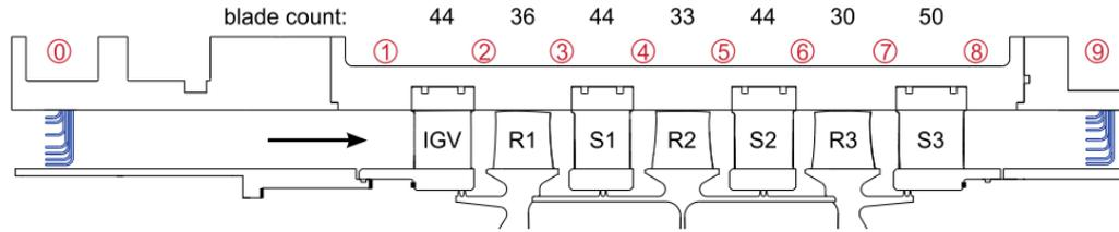
Figure 2 : Purdue 3.5-stage compressor rig. Rotor 2 is mounted with NSMS tip timing and aerodynamic probes.
