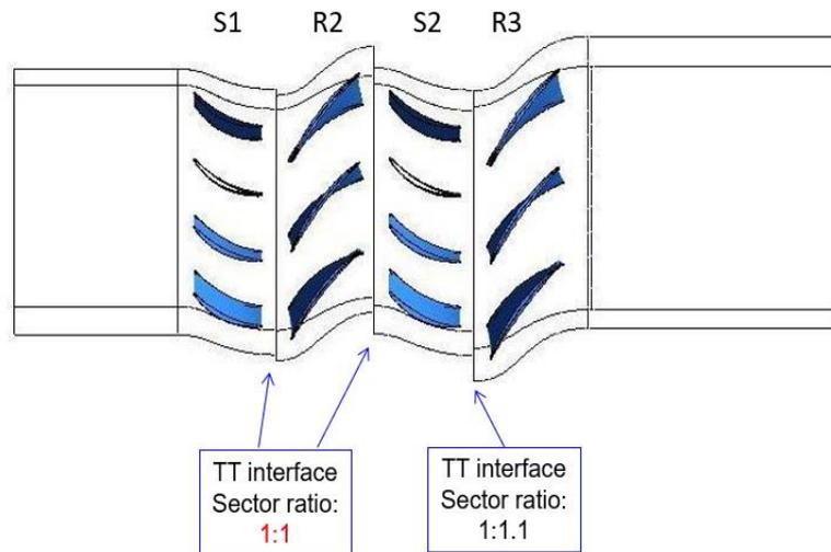
**Figure 6 : Sketch of the 4-row simulations. Sector ratios between different rows are marked in two boxes.**
