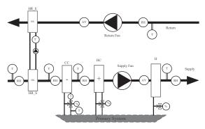
Fig. 2 – Schematic of Aztarain AHUs (Sterling, 2016)
