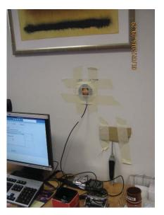
Fig. 4 – Internal measurement equipment for heat flow rate, surface temperature, and air temperature (Passerini, 2016)
