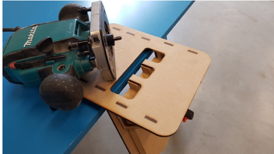
Figure 35. Jig for cutting a finger joint
