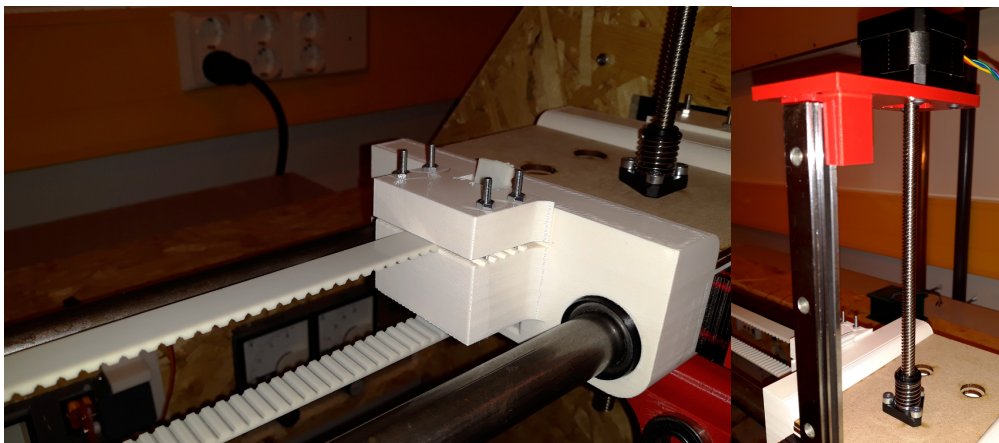
Figure 6: Using toothed belt and lead screw on the second prototype.
