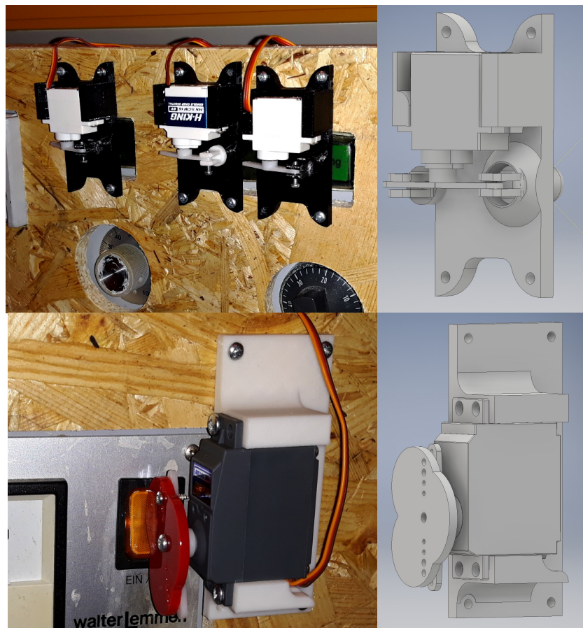
Figure 10a, b: Design and implementation of the modules to control the button (top), rocker switch (bottom).
