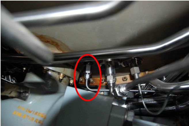
Figure 2 – RB211-24G LP Compressor Discharge Pressure fitting and tubing
