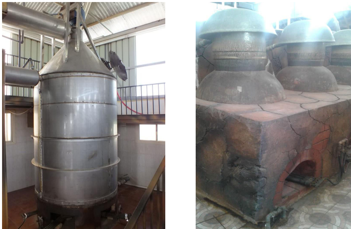
Figure 2. The stainless steel (left) and copper (right) apparatus used for extracting the Rosa damascene Mill
