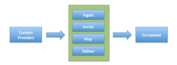
The overall streamline of the above tasks can be seen in the above picture and fall into four main steps: a) content is first ingested into the infrastructure, b) metadata records are enriched through one ore more of the enrichment micro-services, c) metadata are mapped from one of the intermediate schemas supported to the target schema (EDM) and finally d) metadata are exported to Europeana or other interested parties (e.g. Wikis owners who can get an enriched version of their content back).
