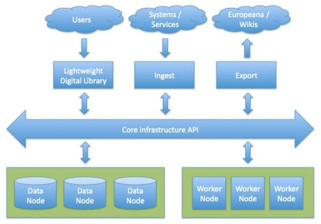
The three interaction points interface with the infrastructure using an API. This core infrastructure API is responsible for maintaining data integrity (e.g. organizing data in packages, per provider/user, etc.), ensuring integrity among versions, maintaining information related with the tasks assigned to each object (e.g. enrichment, mapping, etc.).
