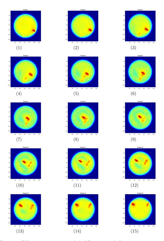
Figure 3: Tikhonov reconstructions of 15 different example frames DataDy-namic\_128x60.mat showing the movement of the cross sections of the aluminum and graphite sticks.
