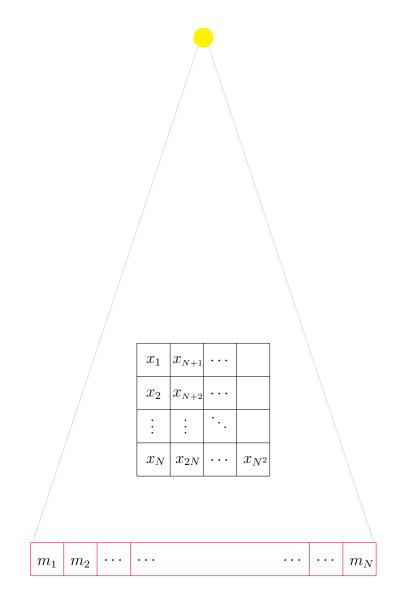
Figure 5: The organization of the pixels in the sinograms  $\mathbf{m} = [m_1, m_2, \ldots, m_N]^T$ and reconstructions  $\mathbf{x} = [x_1, x_2, \ldots, x_{N^2}]^T$  with N = 256. The picture shows the organization for the first projection; after that in the full angular view case, the target takes 6 degree steps counter-clockwise (or equivalently the source and detector take 6 degree steps clockwise) and the following columns of  $\mathbf{m}$  are determined in an analogous manner.
