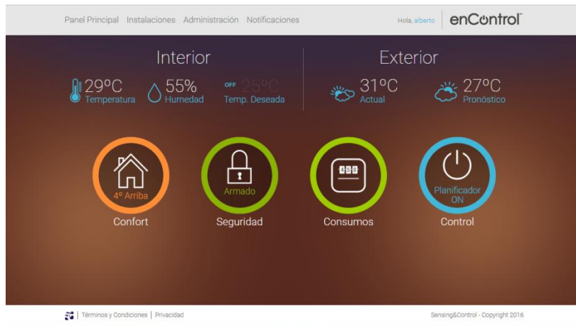
Figure 5: Main screen for all functionalities provided by enControl: comfort, security, energy consumption and automatic control of devices
