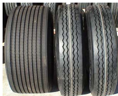
Fig. 7 Single wide base and dual tires [21]
