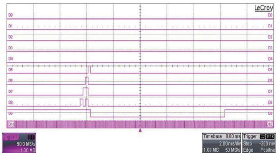
Fig. 4 (c) Results of the FPGA at 51 Hz recorded on a high resolution logic analyzer
