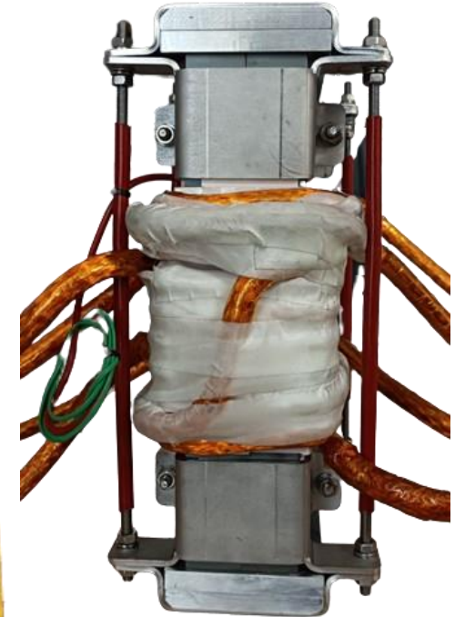
Primary winding perpendicular across secondary winding. Less losses.
