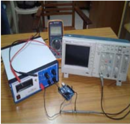
Fig. 9 (b) Testing set up of Arduino Mega 2560
