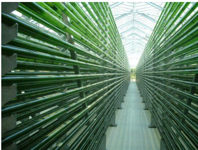
Figure 23 : 500 km long, 600 m 3 tubular manifold PBR in a greenhouse operated by Algenfarm Klötze, Germany
