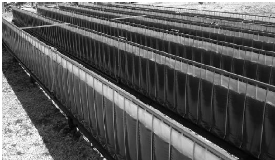
Figure 28 : Green Wall Panel-II photobioreactors at the F&M facility in Siesto Fiorentino (Italy)
