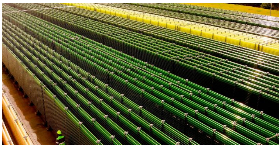
Figure 24 : 1.300 m 3 tubular PBR designed by A4F for Secil/Almicroalgae Algefarm in Pataias, Portugal
