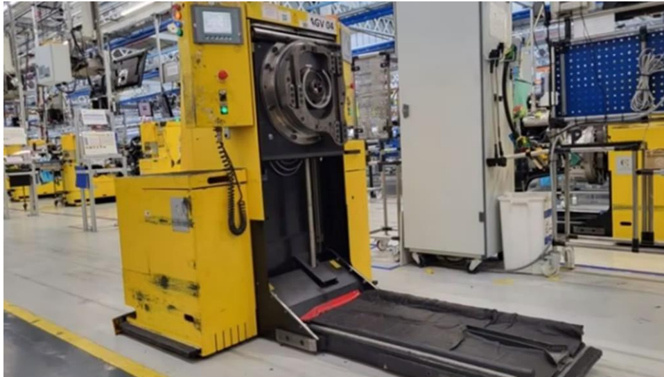
Figure 4: IoT supported AGV fleet by Volvo Group 3
