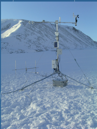
The lower melt and weather station at A.P. Olsen Ice Cap, upon installation in 2008. Photo: Michele Citterio
