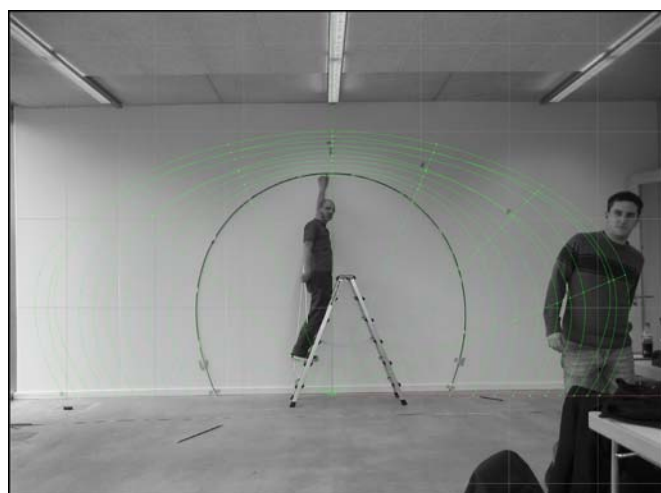
Fig. 2 Reverse Engineering: Photogrammetry of the physical rod-structure in relation to the digital arc-structure
