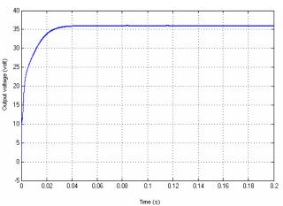
Fig.14 Output voltage when inductor varies from 100μH to 500μH
