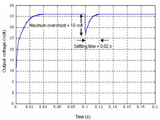
Fig. 9 Output voltage when input takes a step change from 12V to ov
