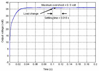
Fig.11 Output voltage when load resistance makes a step changes from 50  $\Omega$  to 40  $\Omega$
