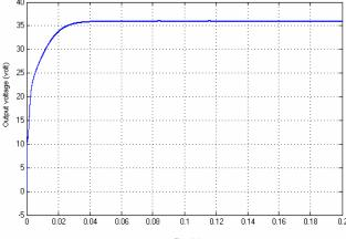
Fig.13 Output voltage when capacitors variation from 30  $\mu F$  to 100  $\mu F$
