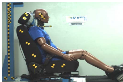
Fig. 5 BioRID II test picture
