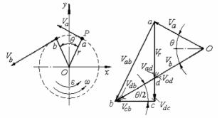
Fig. 1. Acceleration of a rotating point
