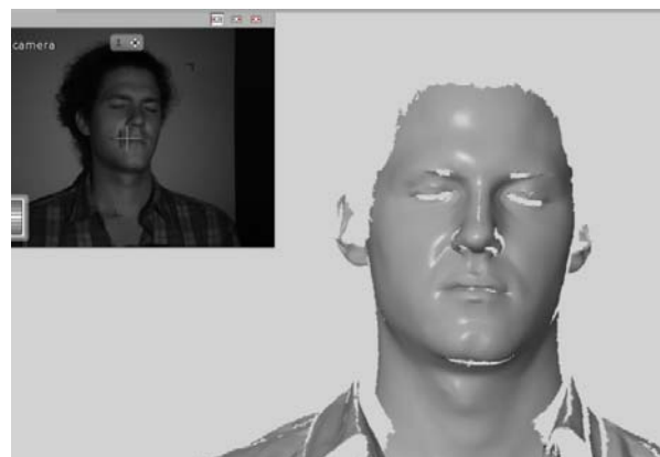
Fig. 11 ATOS I without reference points, 2 snapshots
