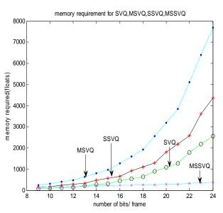
Fig. 4 Memory requirements for 3-part SVQ, 3-stage MSVQ, 2switch 3-part SSVQ, and 3-stage 2-switch 3-part MSSVQ at various bit rates
