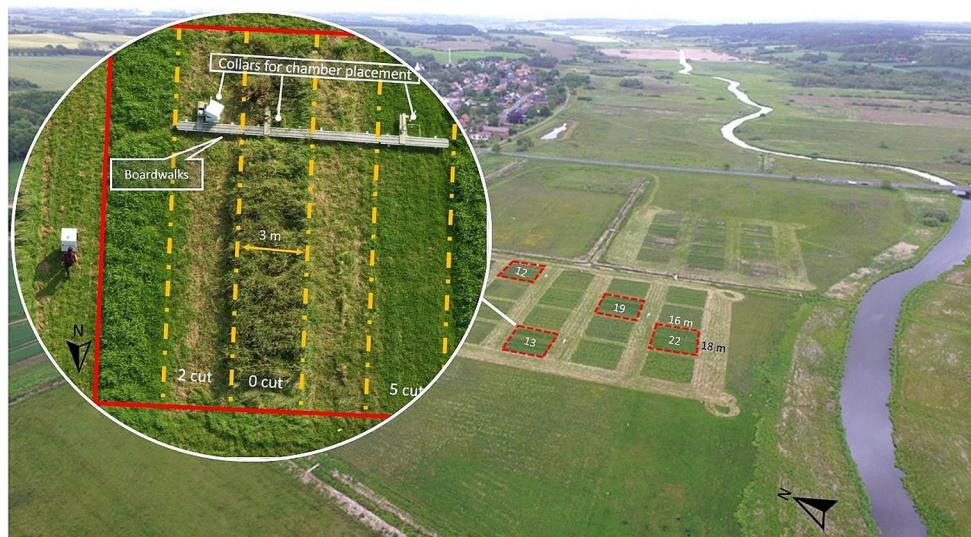
Fig. 1 Drone picture of the Vejrumbro field site in the Nørre Å river valley. Plots used for the field trial are highlighted in red, with plot numbers indicated within the plots. A close-up shows a schematic illustration of the split-plot design, including infrastructure for greenhouse gas measurements. Drone pictures were taken by Jens Kjeldsen
