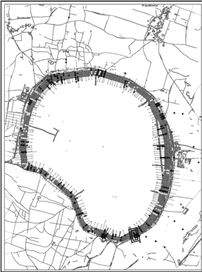
Fig. 3 Plan view of the Želazny Most tailing dam – the black dots show the locations of the CPTs performed and the light grey dots show the locations of the CPTs used in further analysis
