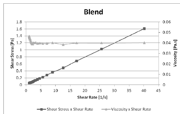
Fig. 6 Blend of vegetable oils flow curve at 40 °C
