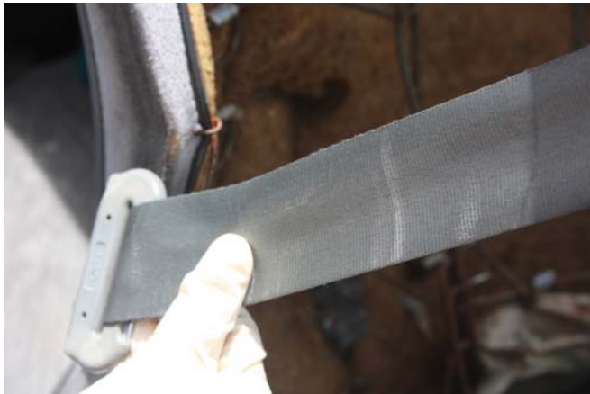
Fig. 1 Abrasive marks indicate physical evidence of seat belt wearing during crash
