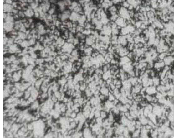
Fig. 1 Optical micrographs (a) base metal (b) heat affected zone and (c) weld metal deposited at a current value of 150A
