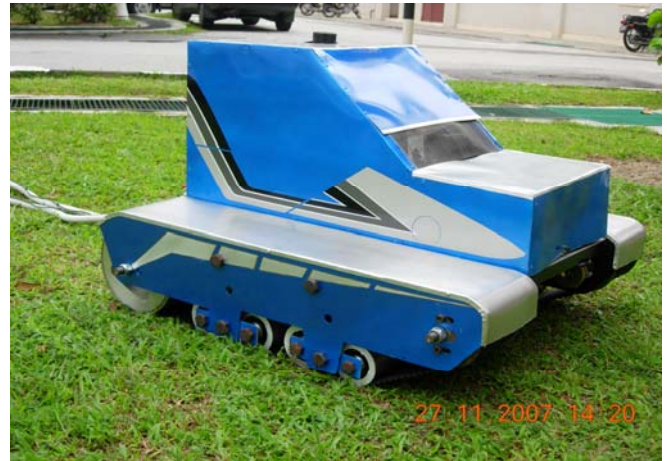
Fig. 6. Developed prototype of air-cushion track vehicle [9]
