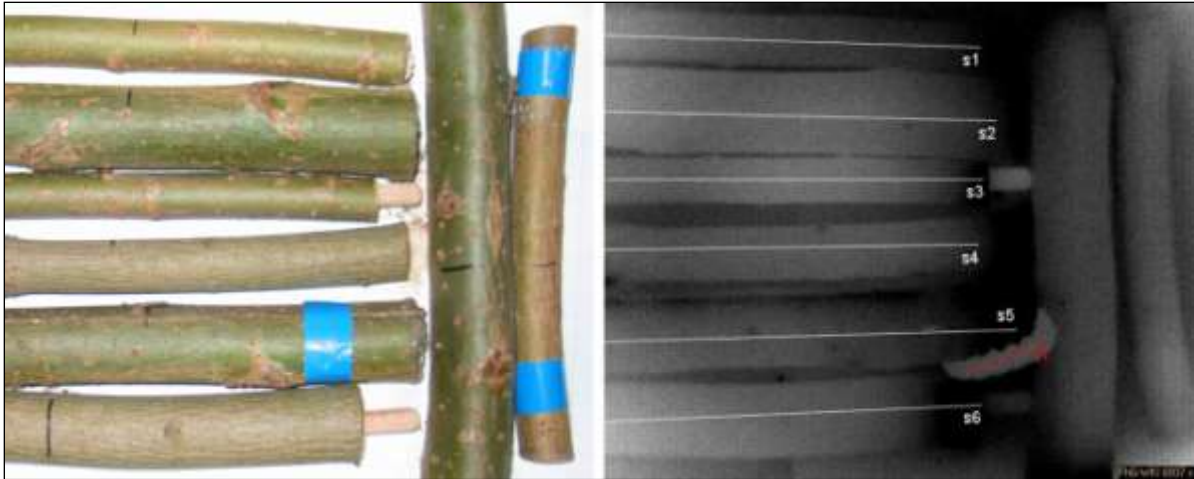
Fig. 15: Thermal test setup of long-term measurement 2. Solid wood samples ( Acer platanoides , Salix caprea ) with axial boreholes in center and inserted Cossus cossus larvae in each sample. Left: Color image with marked positions at the end of boreholes. Right: Thermal image with measurement setup of thermal determination lines (s1 to s6). Test object I1 shows one of two “free” larvae.
