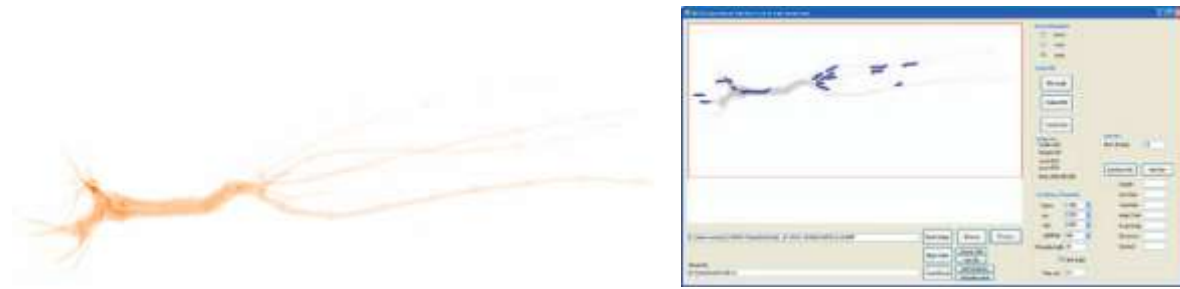
Figure 2-2. X-ray image of an Acer tree infested by Anoplophora chinensis (left) and automated detection of gallery in the stem of the intact tree, marked in blue (right).
