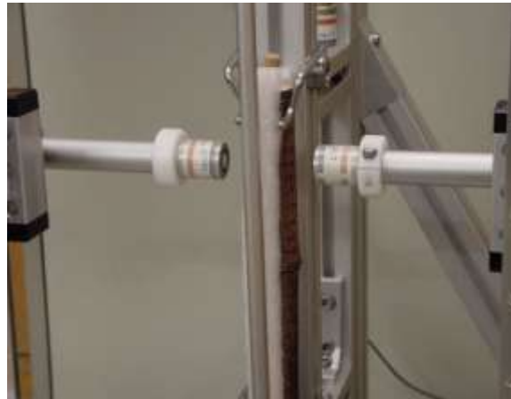
Fig. 25: Air-coupled transducer AirTech 200 and wood sample at scanning process. Foam material reduced wave propagation on the surface of samples.
