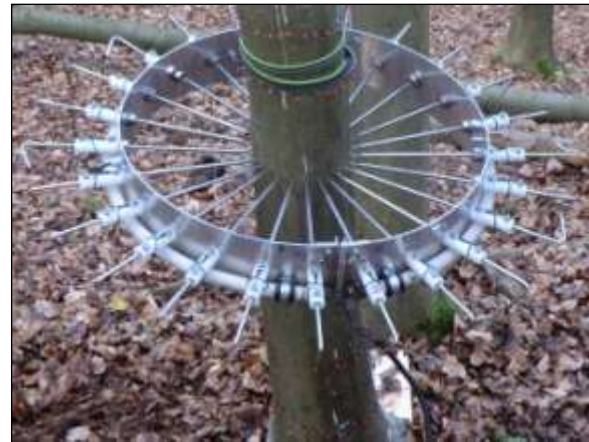
Fig. 5: Configuration-ring of electrodes at standing tree of the University of Applied Sciences and Arts (HAWK) Göttingen/Germany
