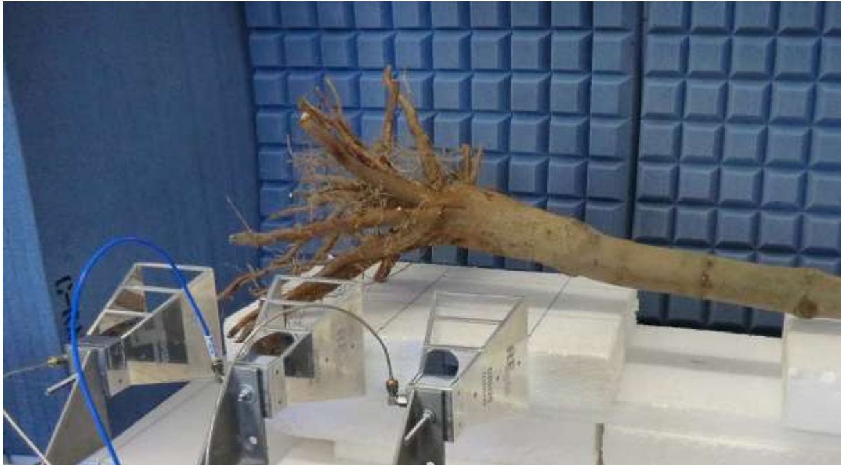
Fig. 17: measurement setup of radar: Three antennas and young tree (root zone)
