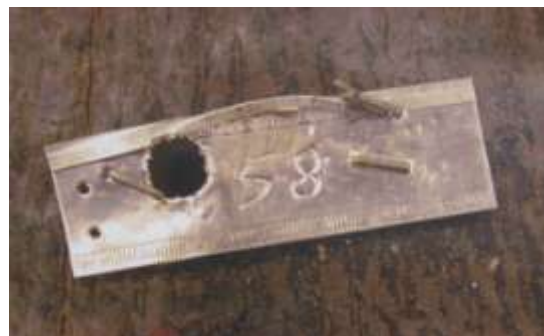
Exit hole through metal tag made by ALB
