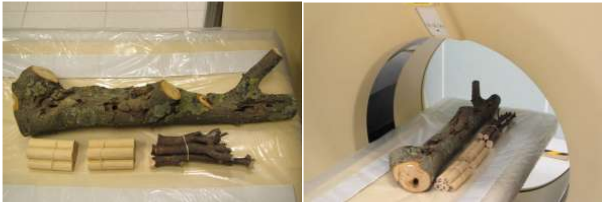
Figure 2-5. Composite phantom for testing the capabilities of CT-imaging of wooden objects: wooden sticks with man-drilled boreholes of 2 and 3 mm , and 2 larger tree branches with a number of substantial boreholes from the long-horned beetle; oven-dried after harvest, and stacked dry at room temperature.
