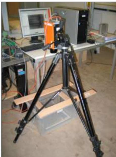
Fig. 14: Thermographic setup for long-term measurement 2
