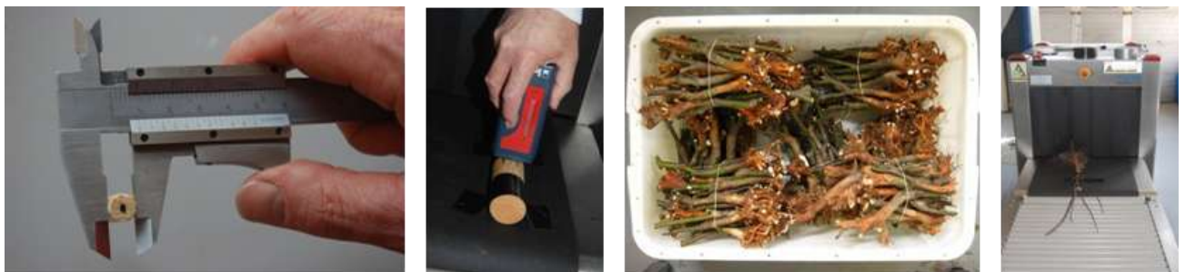
Figure 2-1. Pilot experiment - development and testing of a non-destructive 2D scanning method: 2D X-ray as a detection tool on individual model plants (pre-drilled wooden axles and Acer stems) and intact Acer trees.
