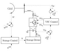
Fig. 1: VSC-based ESS coupled to the grid.
