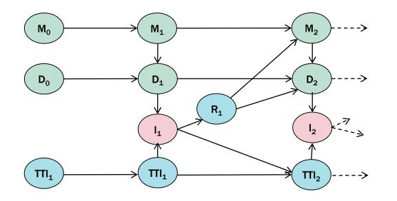
**Nodes / variables** Damage size:  $D_i$ Model parameter:  $M_i$ Inspection outcome:  $I_i$ Preventive repair decision:  $R_i$ Time to inspection:  $TTI_i$
