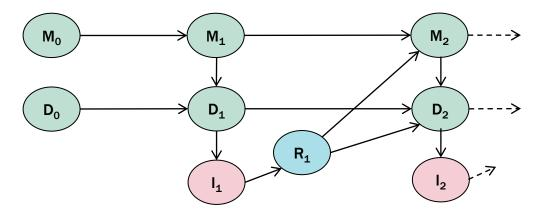
**Nodes / variables** Damage size:  $D_i$ Model parameter:  $M_i$ Inspection outcome:  $I_i$ Preventive repair decision:  $R_i$
