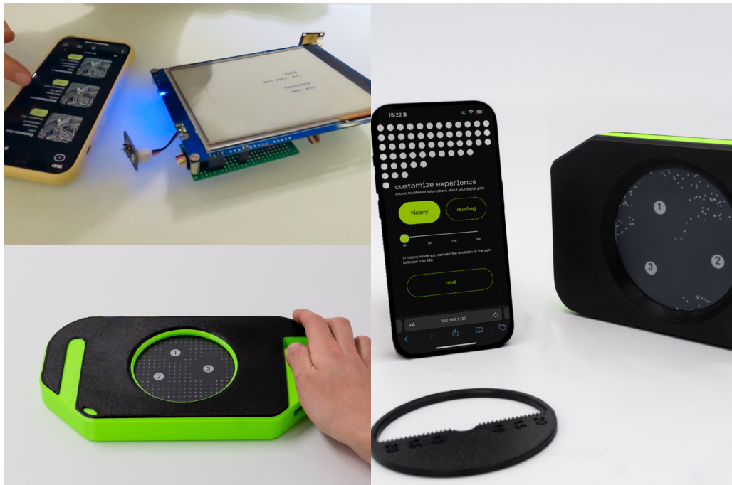
Figure 5: the three versions of DiPLab, the Beta Version (top-left), the first version (bottom-left) and the actual version (right). Image courtesy of MAKEAWARE CC BY 4.0.
