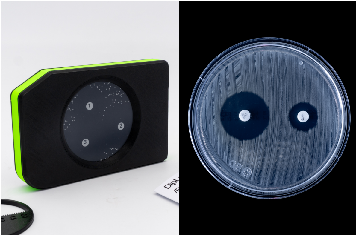
Figure 1: the DiPLab device and petri dish for conducting the Kirby-Bauer test. Image courtesy of MAKEAWARE CC BY 4.0.
