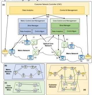
Fig. 1. Management architecture and network slice concept
