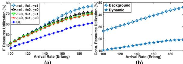
Fig. 5: (a) Average IT resource utilization; (b) Average connectivity resource utilization for  $\alpha = 1, \beta = 1, \gamma = 1$
