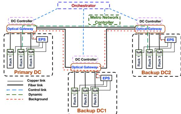
Fig. 1: Proposed control plane for joint resource allocation in converged metro network architecture.
