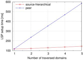
Fig. 5. Simulation results: connection establishment time vs. number of traversed providers.
