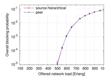
Fig. 3. Simulation results: connection blocking probability vs. offered network load.
