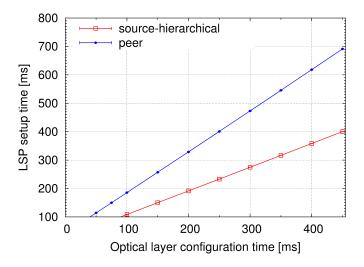
Fig. 4. Simulation results: connection establishment time vs. time required to configure an EON node.
