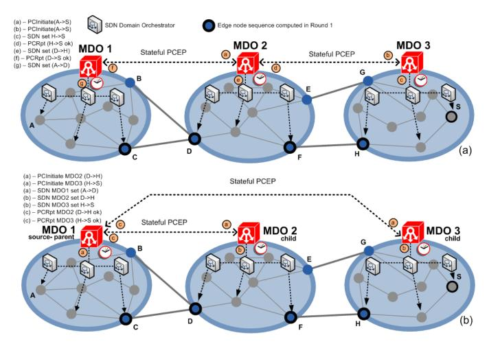
Fig. 1. Proposed architecture: peer (a) and source-hierarchical (b) procedures, for establishing inter-provider connectivity.
