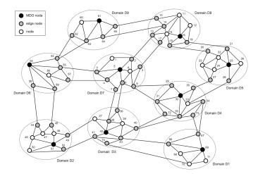
Fig. 2. Multi-provider EON test network topology.
