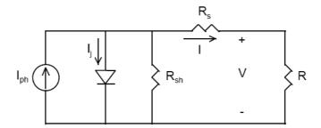
Figure 1: Equivalent circuit for solar cell.
