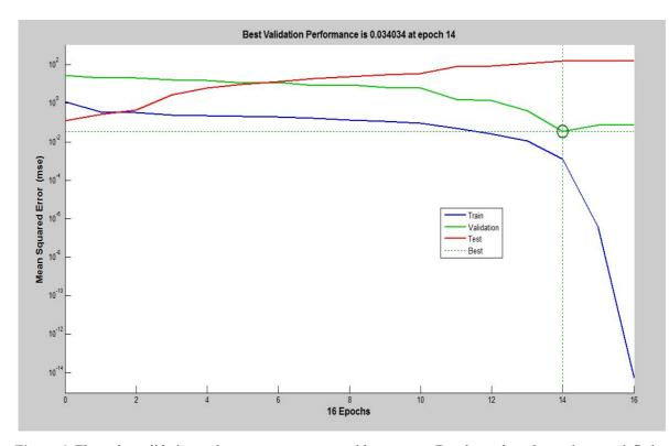
Figure 4: The train, validation and test curves response with respect to Epoch number, the goal was satisfied at 14'Th Epoch.
