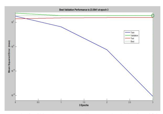
Figure 3: The train, validation and test curves response with respect to Epoch number, the goal was satisfied at 3'rd Epoch.
