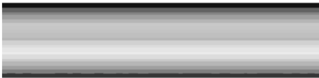
Fig. 5 Initial temperature field for multi-mode film boiling (black - 625 K; light gray - 640 K)
